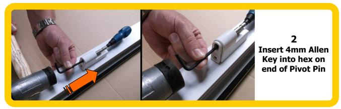
Insert a 4mm Allen Key into the Hex Slot in the bottom of the Pivot Pin. Ensuring that the Screw Driver remains in place, tap the Allen Key into the Pin until the Hinge Body starts to slide off the Frame Mount
