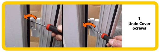
Open the door to access the Cover Retaining Screws. These are self retaining screws therefore to release the cover the screws must be completely unscrewed however the screws do not come out
