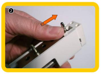
Hinge will normally be supplied unlatched. However, if it is necessary to remove Frame Mount insert flat screwdriver behind metal tang and lever towards Pivot Pin. With screw driver still in place, slide Frame Mount out as shown
