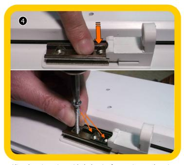
Align location pins with holes in frame, insert the pins and push the Frame Mount fully down.
