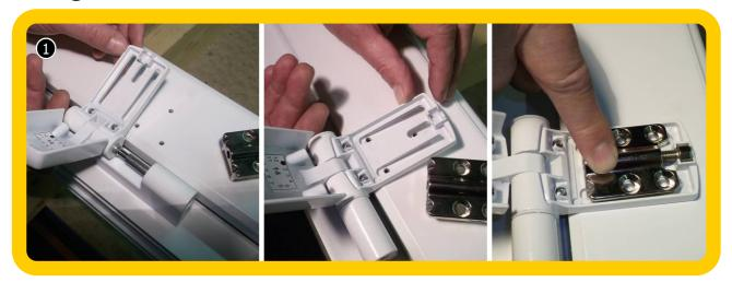
Slide Flag Assembly onto Frame Mount Pivot Pin and push all the way down. Align location pin holes with Sash Plate. Insert the Screw Plate with Location pins into pre drilled holes and push fully down.
