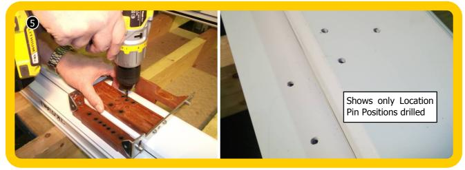
Using a Ø4.0mm drill bit, drill through the skin of the profile only, at the Pin Locations as shown below and as marked on jig. Note: only drill Left or Right Hand pin locations as required when drilling the frame side. If not using drill point screws continue to pilot the remainder of the holes as required
