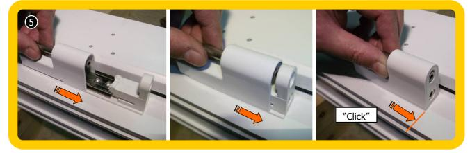
Slide Frame Body casting onto Frame Mount and push all the way down until it clicks into place and until it is flush with the bottom of the Frame Mount Moulding
