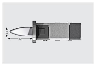
Specially designed twin nickel plated alloy deadbolts are chamfered to allow a high degree of fitting tolerance for door installation. In addition, the deadbolt shape provides low operating forces and helps doors achieve a higher level of weather performance.
