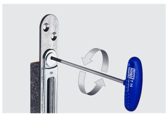
Keeps fully adjustable ±2mm utilising the Torx T15 adjusting tool.
