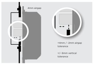
Diagram shows the increased tolerances for door installation using a  $\,^{\text{\tiny TM}}$
