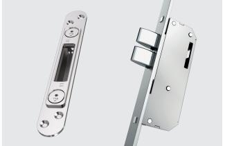
Utilises the same keeps as the popular Winkhaus Cobra™ and Trulock™ range of locks. The split twin deadbolts help to distribute abusive loads and have been tested up to 6.5Kn force, 45% greater than the requirements of PAS24.
